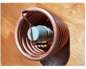
Connecting the trap between the input and output pins of the miniVNA makes the final adjustment of the spacing of the turns to get the trap centered within 30 meters easy.
