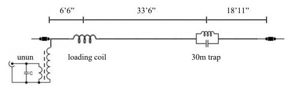
The antenna was constructed of 14 AWG stranded wire with PVC insulation. The loading coil is made by just passing the wire through drilled holes in a piece of 3 inch diameter PVC pipe. I made the coil with 10 turns to begin with but ended up removing a turn to shift the 20 meter SWR minimum point up as needed. 9 turns gives 6.5 uH inductance. The excess wire from the unused turn was removed at the end where the unun matching device is attached.
